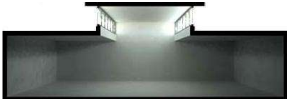
Figure 34: Daylight strategy – Monitor aperture (Source: ECOTECT Community)
