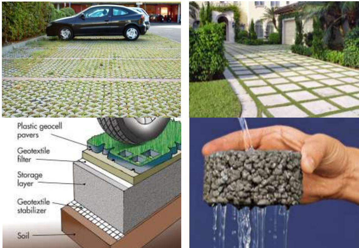
Figure 21: Commonly pervious materials for sidewalks and roads
