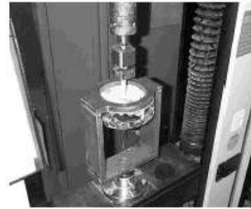
Figure 3 – A test setup for pullout testing.
