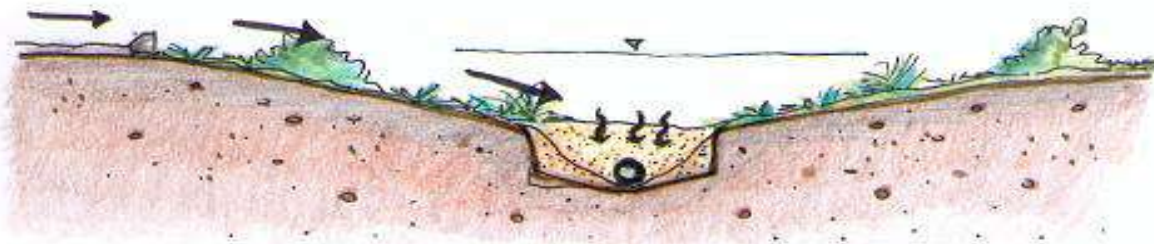
Figure 22: Stormwater management - retention pound (Source: Centro de aguas urbanas)
