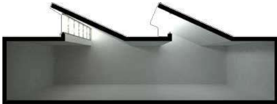
Figure 33: Daylight strategy – Saw-tooth apertures (Source: ECOTECT Community)
