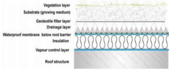
Figure 73: Section of a typical green roof system
