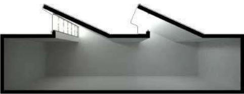
Figure 33: Daylight strategy - Saw-tooth apertures (Source: ECOTECT Community)
