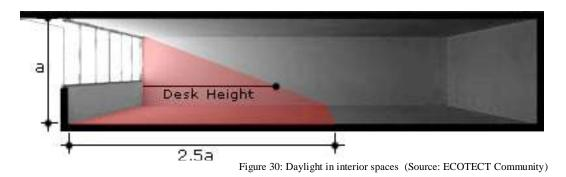
To improve daylighting within a building, windows can be added on multiple sides of the room, or a distribution system such as a lightshelf or prismatic glazing can be used to direct some of the light up onto the ceiling where it will diffuse deeper into the space.
