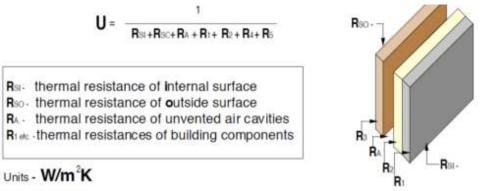
Figure 44: U value diagram (Source: architecture.com)
