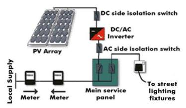
Figure 62: Grid-connected photovoltaic power system diagram
