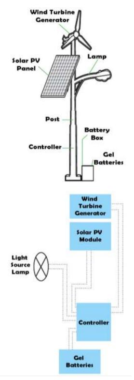
Figure 61: Hybrid lighting system diagram
