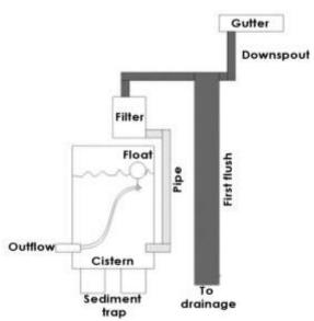
Figure 65: Main components of rainwater harvesting systems
