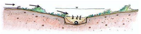
Figure 22: Stormwater management - retention pound (Source: Centro de aguas urbanas)
