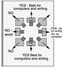
Figure 27: Interior distribution and daylight (Source: WBDG)
