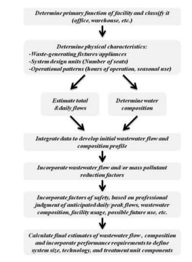
Figure 66: Methodology for estimating wastewater resources and proceed to an adequate selection of treat ment systems
