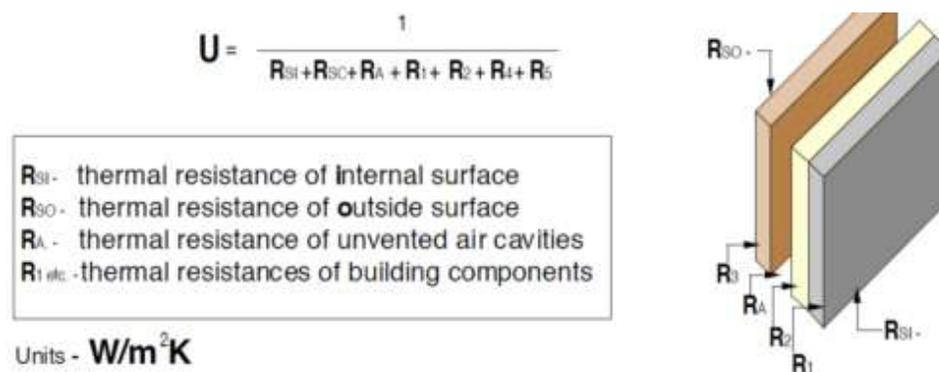
Figure 44: U value diagram (Source: architecture.com)
