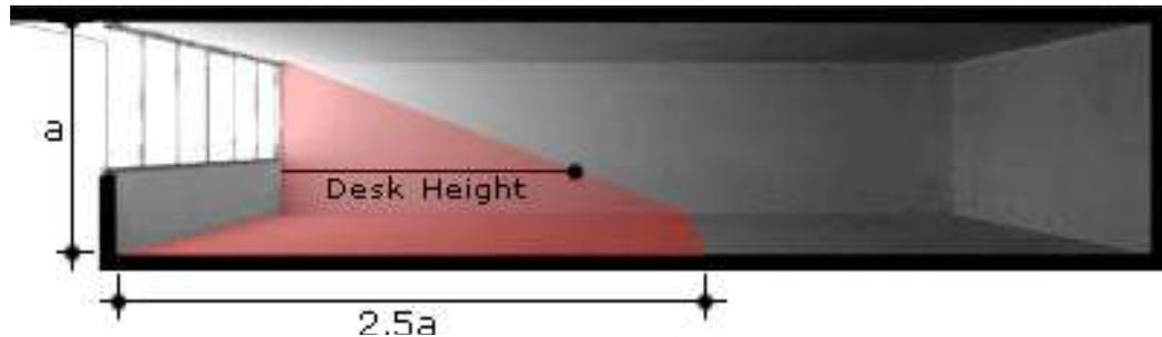
Figure 30: Daylight in interior spaces (Source: ECOTECT Community)
