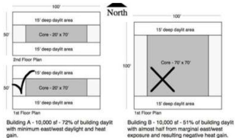
Figure 29: Daylight and building shape (Source: WBDG)
