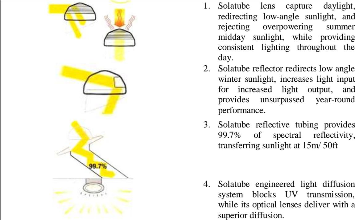
1. Solatube lens capture daylight, redirecting low-angle sunlight, and rejecting overpowering summer midday sunlight, while providing consistent lighting throughout the day.
