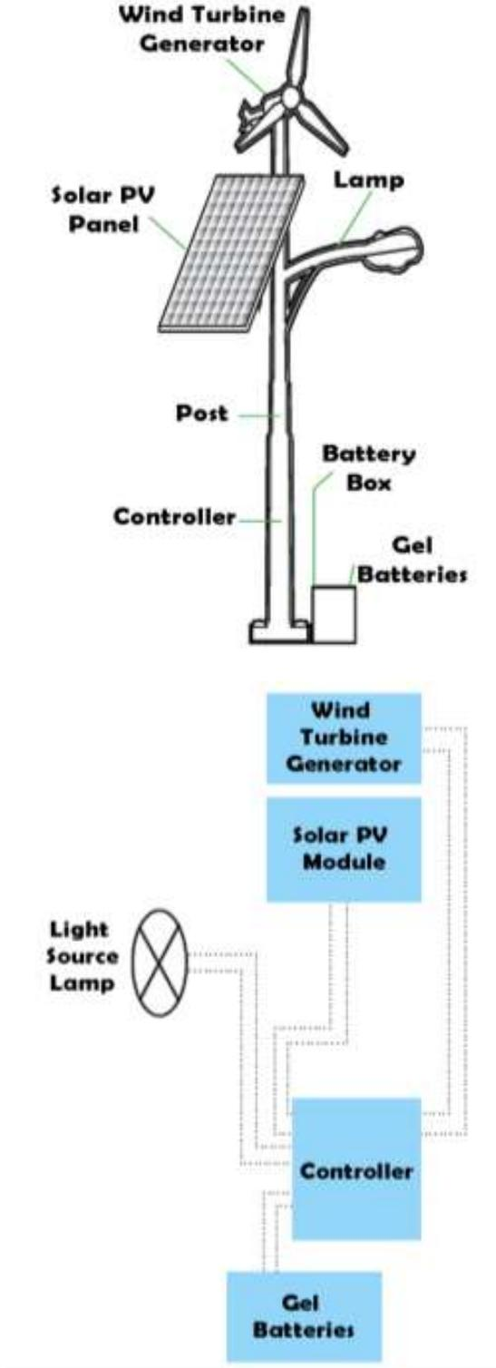
Figure 61: Hybrid lighting system diagram
