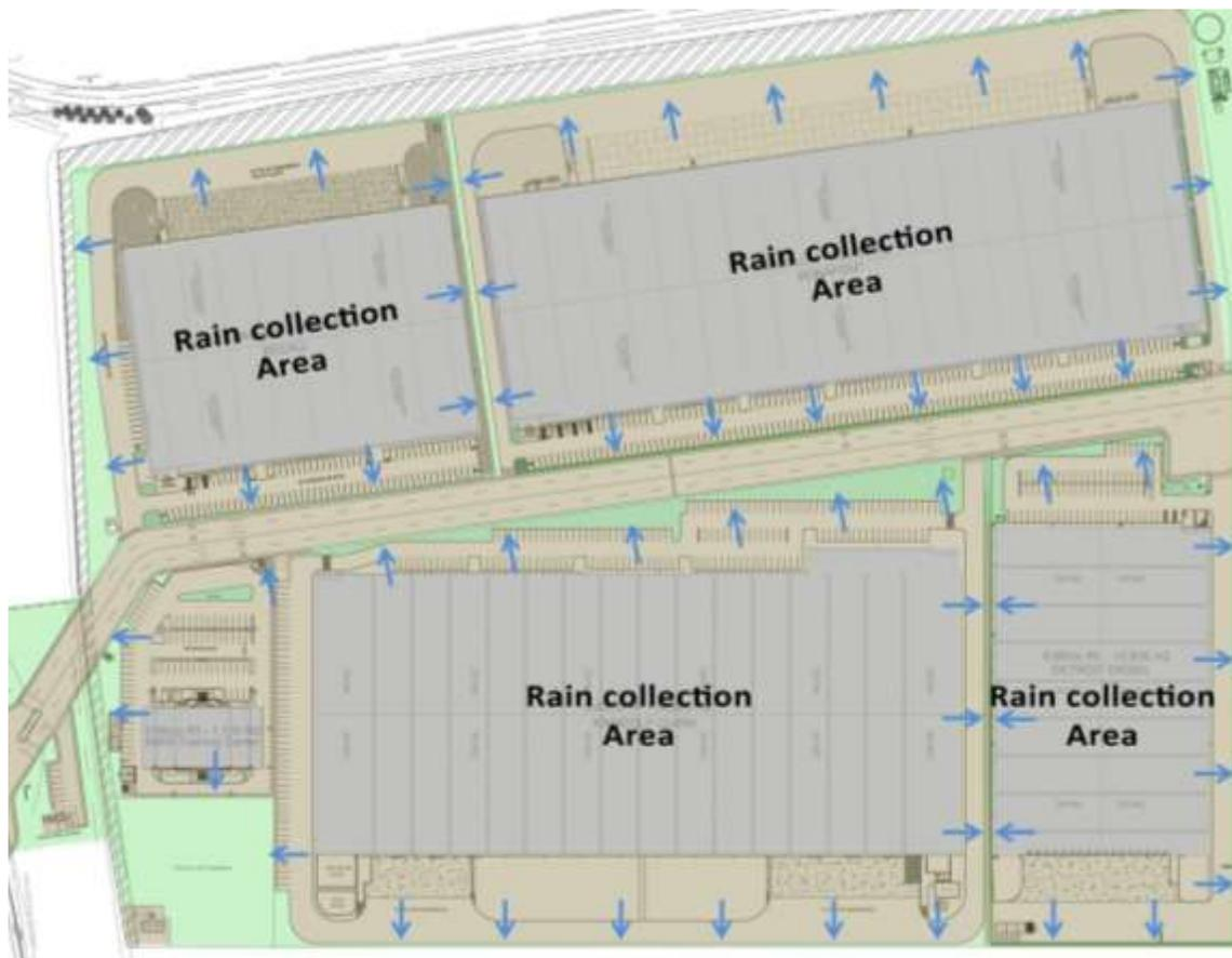
Figure 64: Rainwater falling on roads should be conducted to green areas
