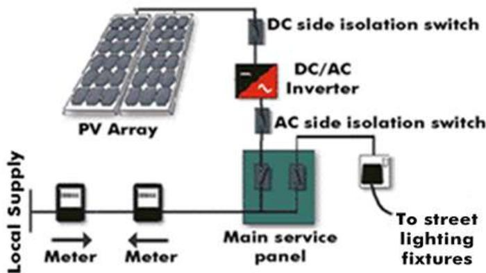
Figure 62: Grid-connected photovoltaic power system diagram
