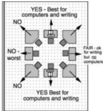
Figure 27: Interior distribution and daylight (Source: WBDG)
