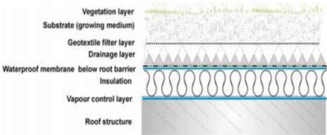
Figure 73: Section of a typical green roof system
