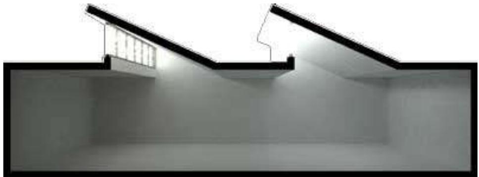
Figure 33: Daylight strategy – Saw-tooth apertures (Source: ECOTECT Community)
