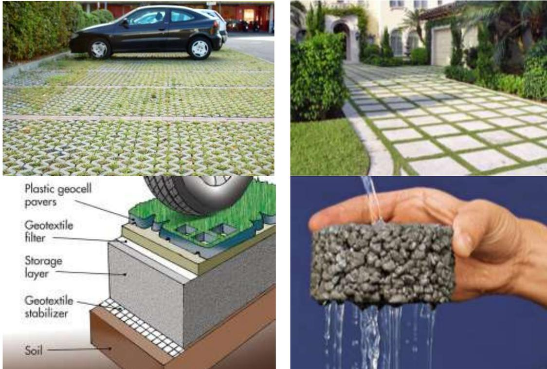
Figure 21: Commonly pervious materials for sidewalks and roads
