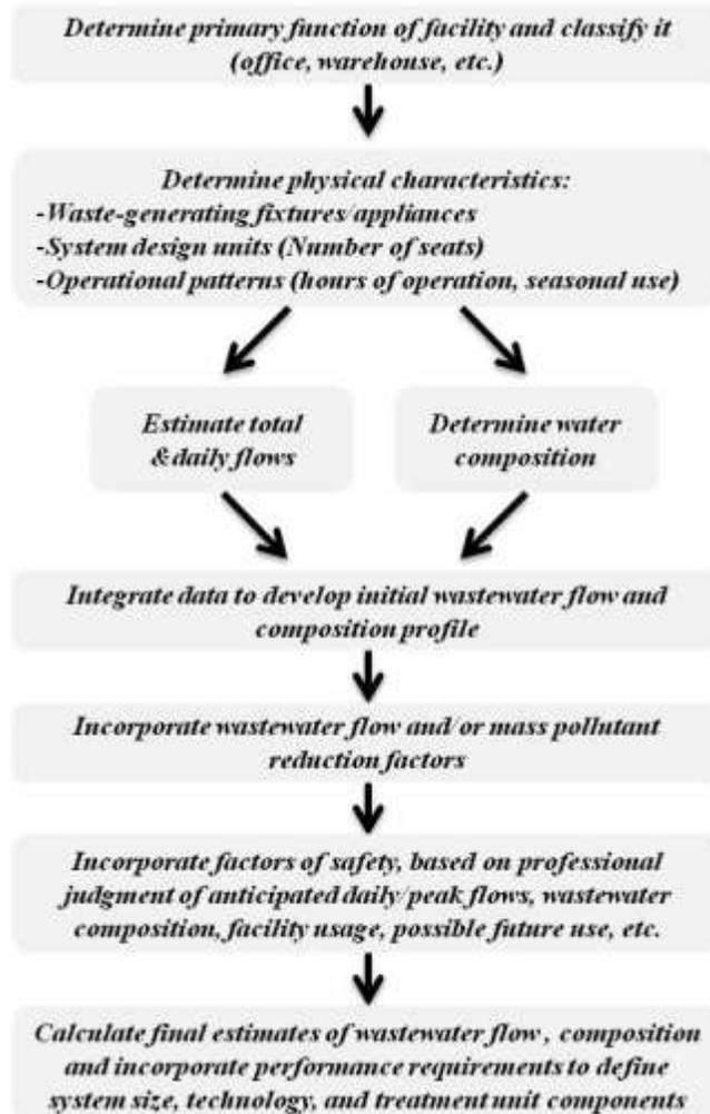
Figure 66: Methodology for estimating wastewater resources and proceed to an adequate selection of treatment systems
