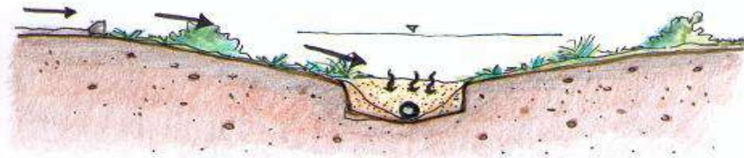
Figure 22: Stormwater management - retention pond (Source: Centro de aguas urbanas)
